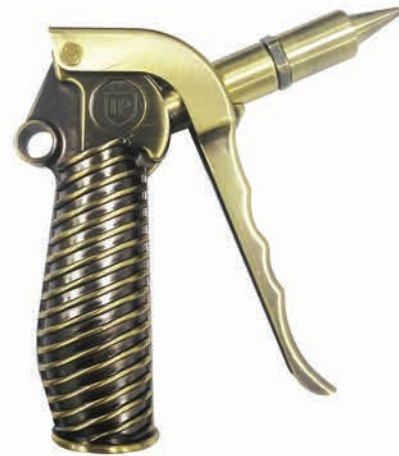
Die Casted Aluminum Heavy Duty Blowgun Copper Plated with body ridges with 3/8" NPT inlet
